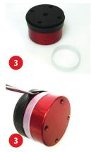
4) Secure AirPuck™ to the bottom of the socket by connecting external hardware into the four hole pattern of the AirPuck™. Make sure the attachment screws do not thread into the puck body more than 13mm (1/2"). The thread holes do not penetrate the Puck interior. Tighten opposite screws to pull the puck down into the void evenly.
