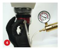
NOTE: Do not disconnect the vacuum source until the valve is closed.
